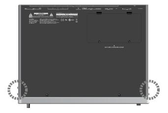
3. Attach the rackmount brackets using the screws you removed in step 2.
